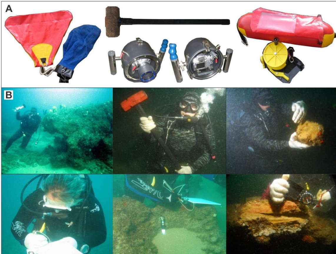
Dive sampling methods. (A) Tools for underwater mapping include a lift bag and net, 14-pound sledgehammer, camera protected in an underwater housing, and a watertight float for a GPS. (B) Photographs of sampling and observation of submerged geological features.
